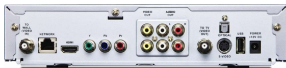
Figure: Typical STB rear panel
