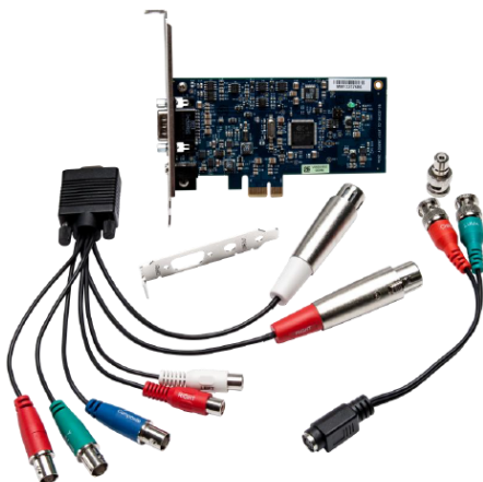
Figure: Osprey 260e and breakout cable
