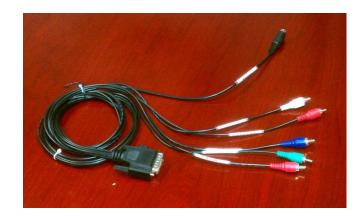
Figure: Breakout Cable Component, Composite and S-Video (Volicon)
