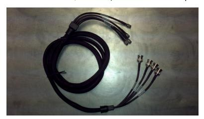
Figure: BNC to Mini BNC Adapter Cable
