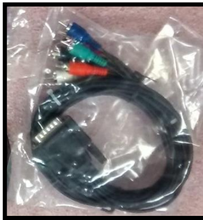
Figure 6.5. Analog Adapter (Breakout cable).
