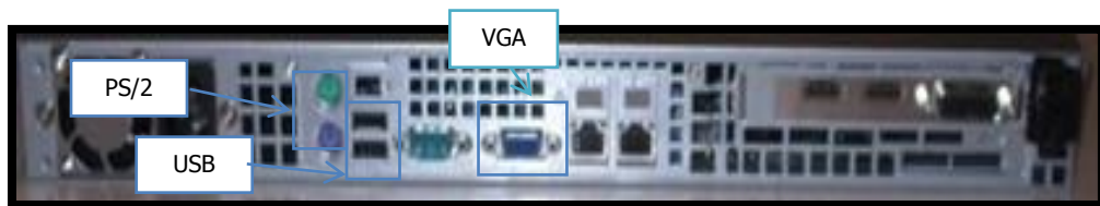
Figure 8.1.1. Volicon Scout Rear View – VGA, USB, & PS/2 locations.
