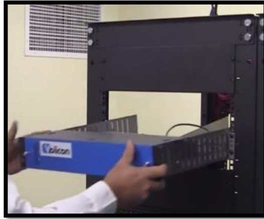
Figure 4.9. STB Shelf Assembly – Rack Installation.
